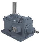
**Gearbox**—Confirm sufficient gear oil and operate the motor for at least five minutes each week to permit internal gear surfaces to be bathed in oil. The fans can be manually rotated to achieve this same purpose if the motor is not hooked up to a power source. Another option is to completely fill the gearbox with a corrosion preventative oil during the shutdown/storage time (and to remember to take it out prior to startup).
