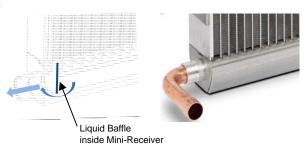
Proper coil orientation and Refrigerant INLET and OUTLET is required. Orienting the coil upside down will result in loss of capacity and high condensing temperatures.
